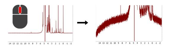
2) Press "b" or click on the red arrow on the bottom of the "Auto Baseline Correction" icon: AutoBaseline Correction..." Select different methods under "Method" and look at the **blue baseline** that has appeared along the bottom of the spectrum. Try adjusting the method-specific parameters for each.
