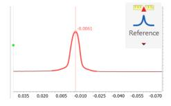
Referencing on a solvent peak is an alternative to using an internal standard (table 1 from this <u>reference</u> can be used for this), but it is generally less accurate because solvent peak shifts are more variable with sample conditions (temperature, acidity, etc.).
