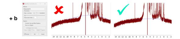
3) A good baseline will be smooth and not contain any bumps. When subtracted, it should center the signal-free regions of your spectrum about 0 on the y axis without causing any dips in your spectrum below zero. (**NOTE:** you may find you need to touch up the phasing to get an acceptable baseline.) Select an appropriate baseline correction method and apply it by pressing "OK." Which did you select?
